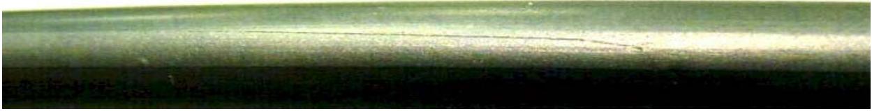
FIGURE 8. ROLL CRACK MARK ON STEEL BAR (CASE A).
