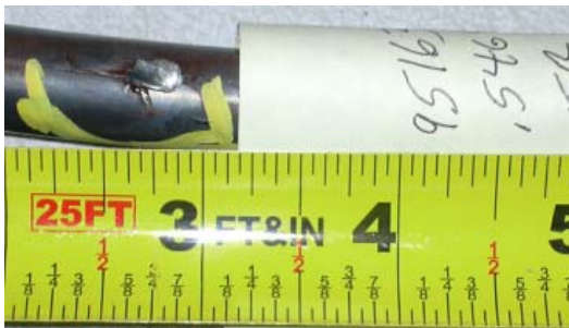
FIGURE 12. SHEARING AND SCAB MARKS DETECTED HOTEYE™.
