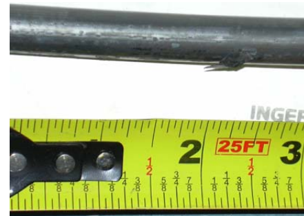
FIGURE 12. SHEARING AND SCAB MARKS DETECTED HOTEYE™.
